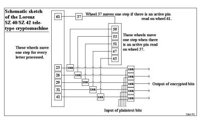
Figure 2: SZ-40 Wiring diagram
