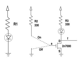
Figure 1: LED Figure 2: NMOS NOT circuit
