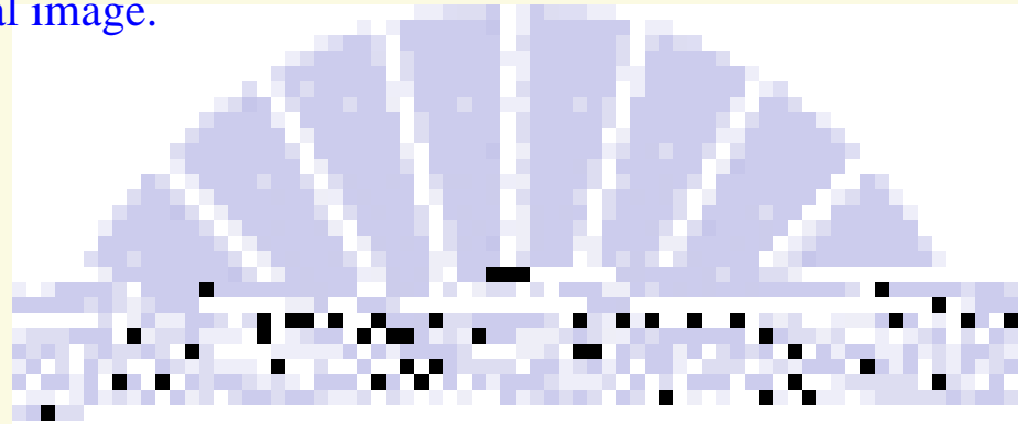
Compressed after FDCT and quantization processing but without entropy encoding
